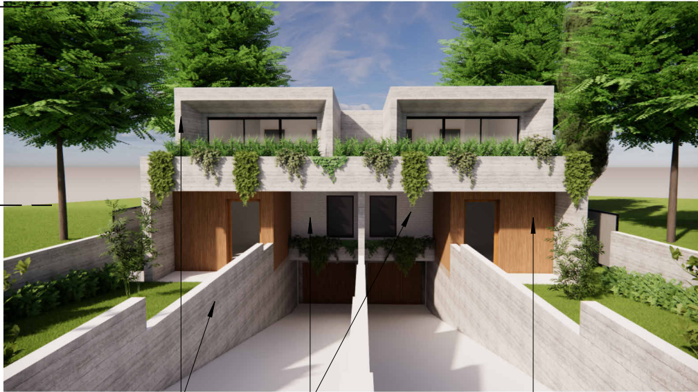
Fair-Faced Concrete White Brick Timber Battens
